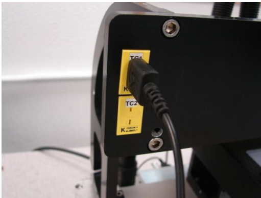
Image 52. TC1 and Fixture Probe Connection
