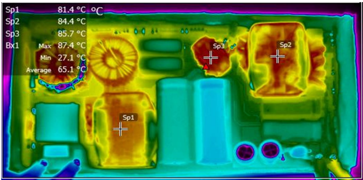
Fig. 12: Topside thermals, 90 V AC , 100% Load (with TIM and copper plate, t AMB =25°C).
