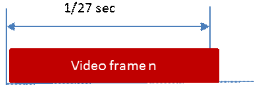
Figure 27 -Clock Too Slow - Failure to Read an Entire Frame Within the Frame Period
